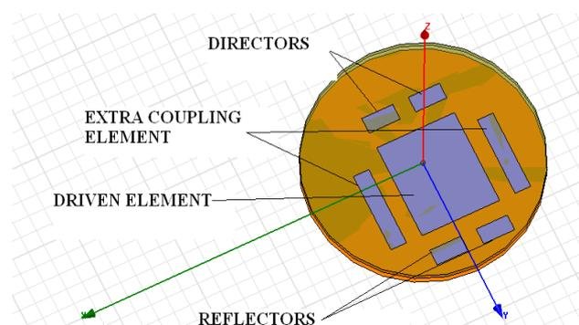
Fig3. Proposed yagi microstrip antenna
